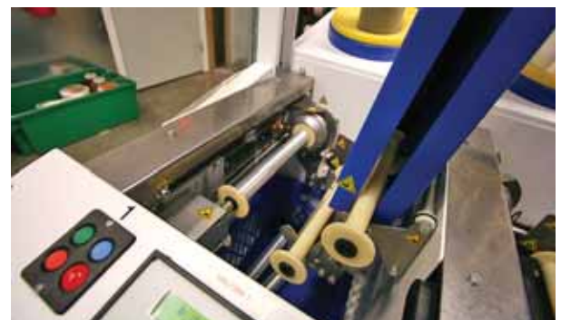
D-P's customized winding machines give a high degree of tension control and consistency when creating super-low-stretch yarns
